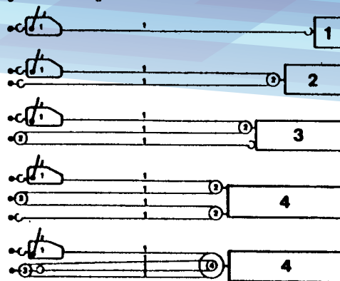
Fig. 8.2 - Lifting by means of reversing sheaves
