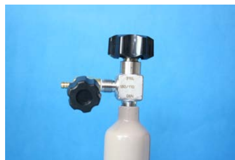
Control valve designated for mildly corrosive or high-purity gases to meter the flow of gas. WARNING: Gas-control valves do not control pressure in a closed system. Regulator or relief valves should be used to prevent the buildup of unsafe pressures that could lead to explosion.
